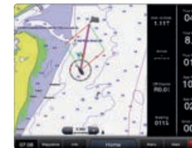
Sailing features: laylines, COG, true wind/apparent wind data displayed at the same time, etc.
